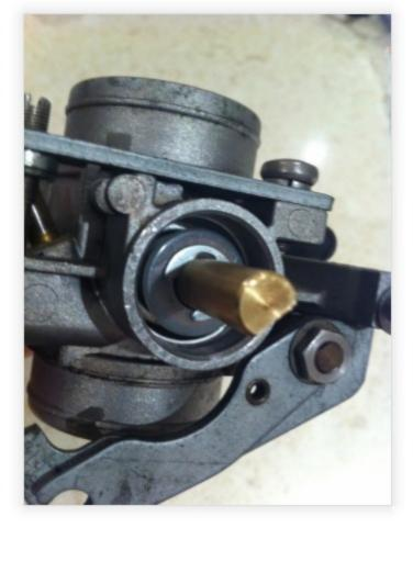
The throttle cam should move fully through its motion without binding and all three butterfly valves should be nearly closed.
